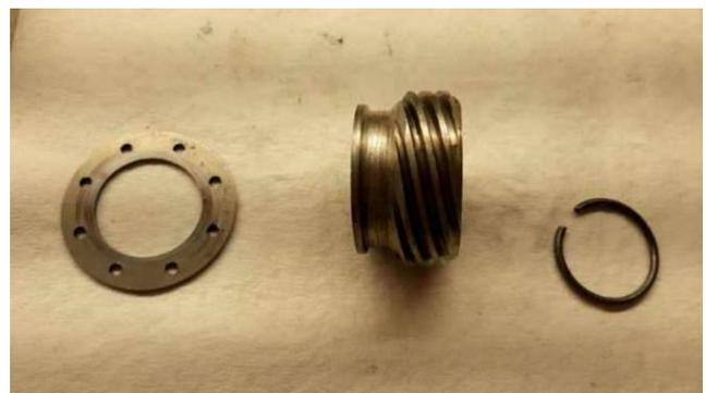
Thrust washer with holes in it slides 1<sup>st</sup> onto the spline shaft, then the speedometer drive gear, and then the keeper ring.
