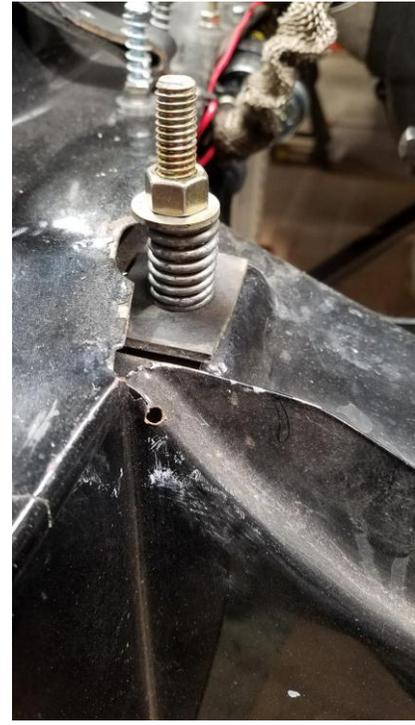
Radiator bolt assembly held in place w/magnet
